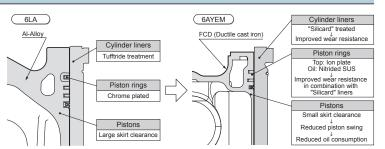
\*\* SiliCard is a surface treatment that uses a special method to embed powdered Silicon Carbide (SiC), an artificial ceramic second only to diamond in hardness, to provide superior wear resistance and durable
