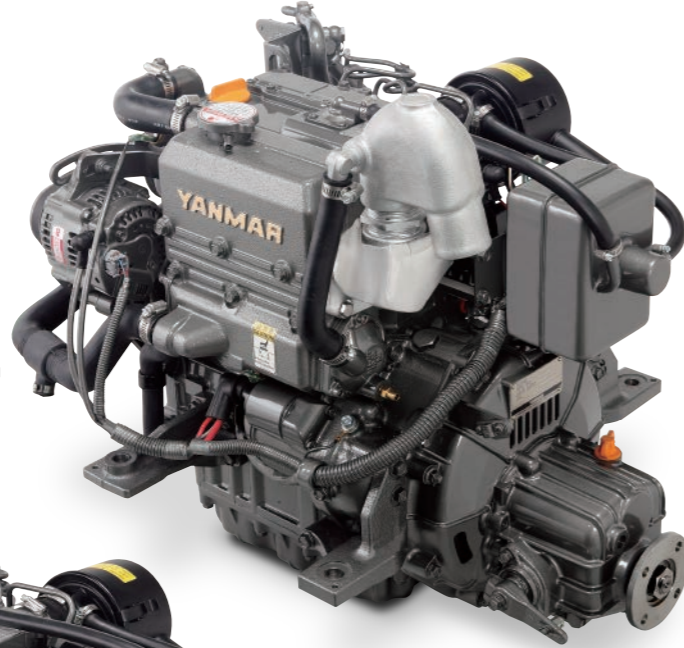
Fresh water cooling with sea water cooled heat exchanger 用海水冷却式换热器进行淡水冷却
