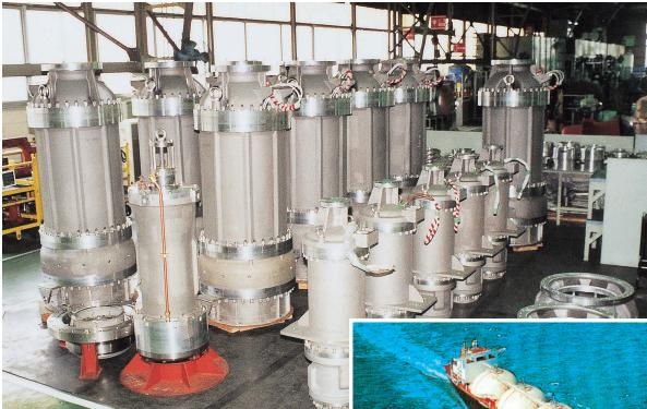
Shinko-Nishishiba LNG/LPG submerged motor pumps are used in many storage stations. And, the cargo pumps for LNG/LPG tankers are also installed on a large number of ships.
