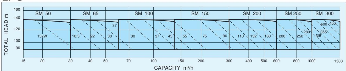
Figure in the chart shows output of motor ( Specific gravity:0.61 )
