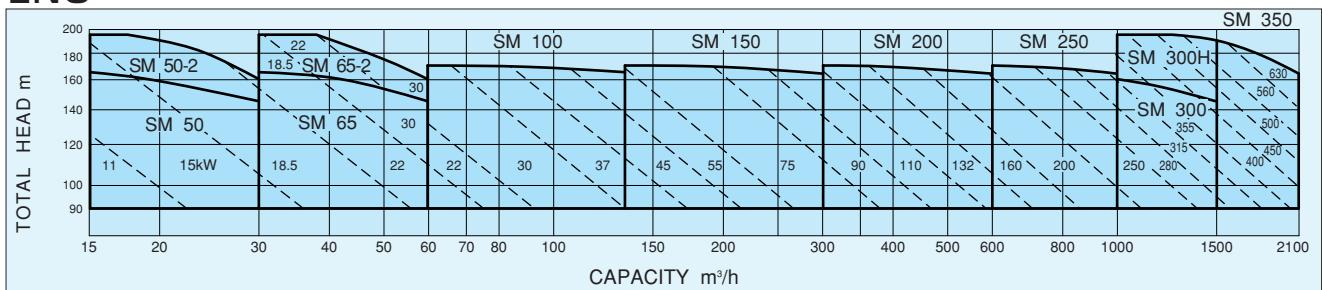
Figure in the chart shows output of motor ( Specific gravity:0.5 )
