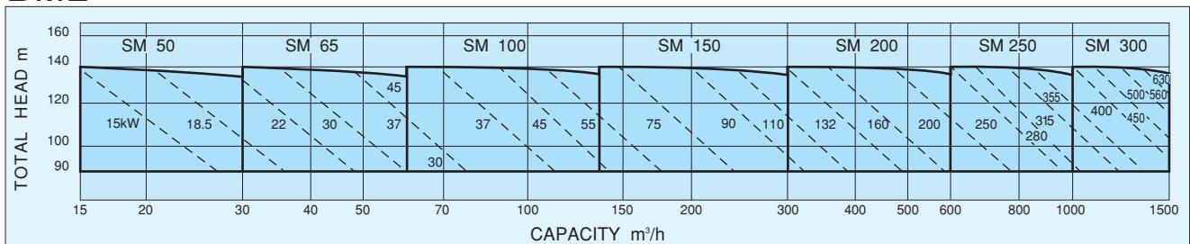
Figure in the chart shows output of motor ( Specific gravity:0.73 )
