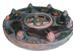
stage valve of a water-cooled compressor after 800 hours
