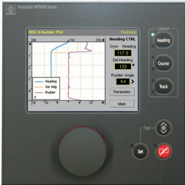
Rudder activity and heading changes are displayed. Autopilot settings can directly be changed.
