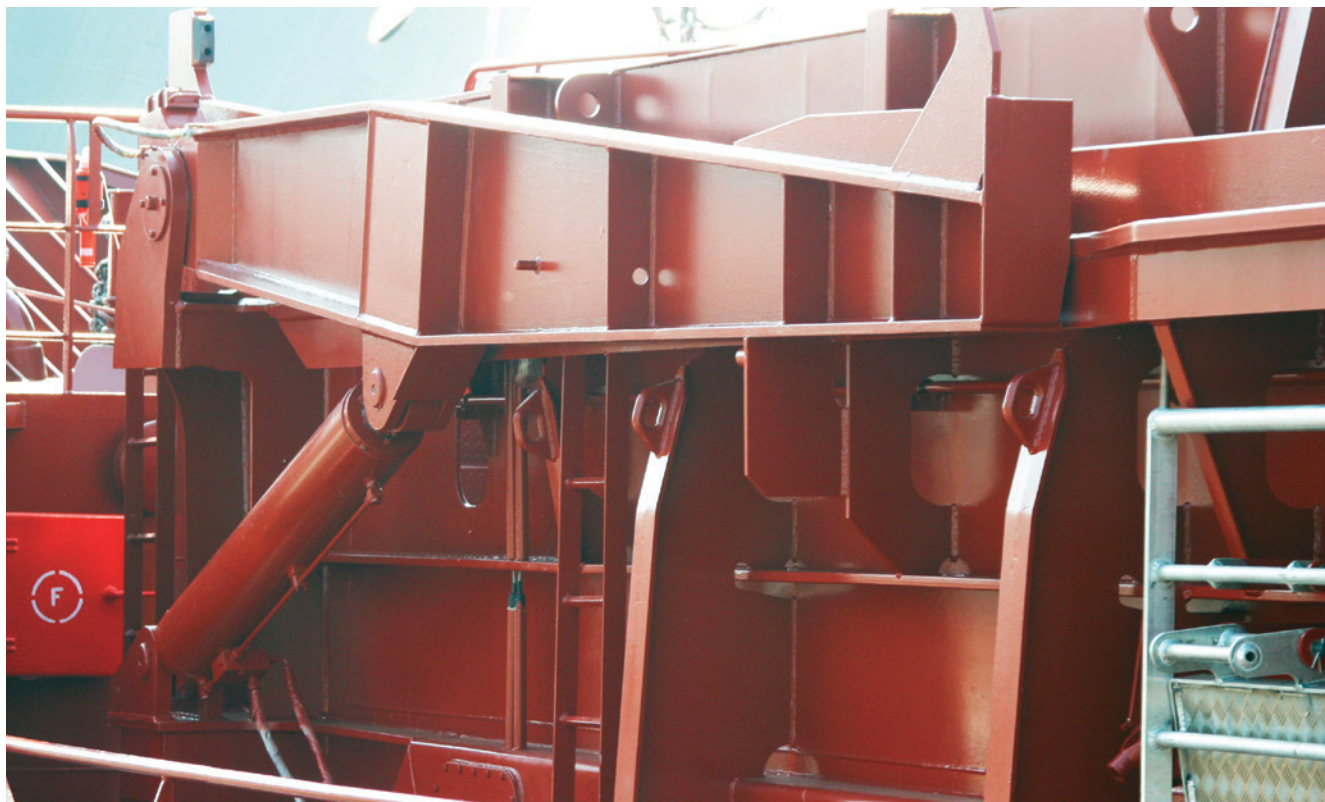
Below: Drive system with cylinders
