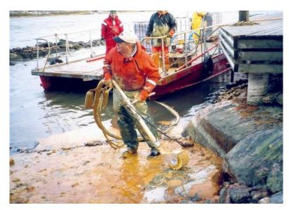
The Rock Cleaner LRC is a hand-held suction nozzle with an integrated brush wheel for improved oil recovery efficiency. It is specifically designed for use on rocky shorelines, in harbors, at oil terminals, ditches, roads, factories, airports and vessels.
