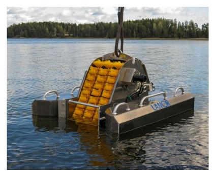
The Multimax LAM 50 is a brush chain-type free-floating oil skimmer designed to recover oil in fast flowing rivers, oil ponds, harbors or as an advancing side sweep skimmer. The skimmer can be used in all terrains and environments, including Arctic conditions.
