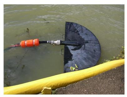
The Rigid Manta Ray is a special weir suction head designed for oil recovery. The skimmer is suitable for thin oil slicks under relatively calm conditions where small debris is present in e.g. lakes and slow moving rivers.
