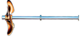
Type A - Propeller and intermediate shaft connected by integral flanges.
