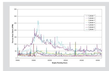
This chart shows the ability of LinerSCAN to detect and trend the amount of iron particles in the cylinder oil in real time.
