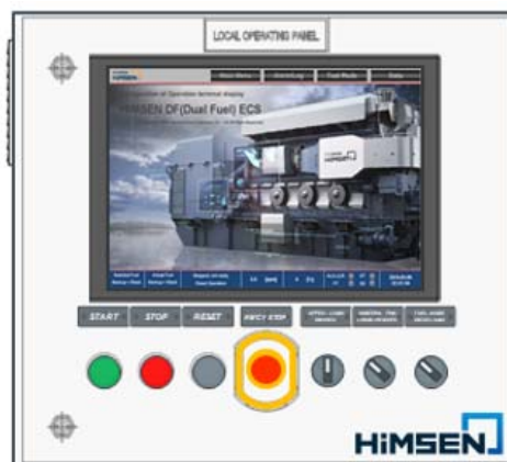
Figure 4-2-4 Local Operating Panel
