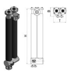
ing medium flows in the surrounding shell. This design allows to compensate for the different thermal expansion between shell and inner tube bundle caused by high temperature differences.
